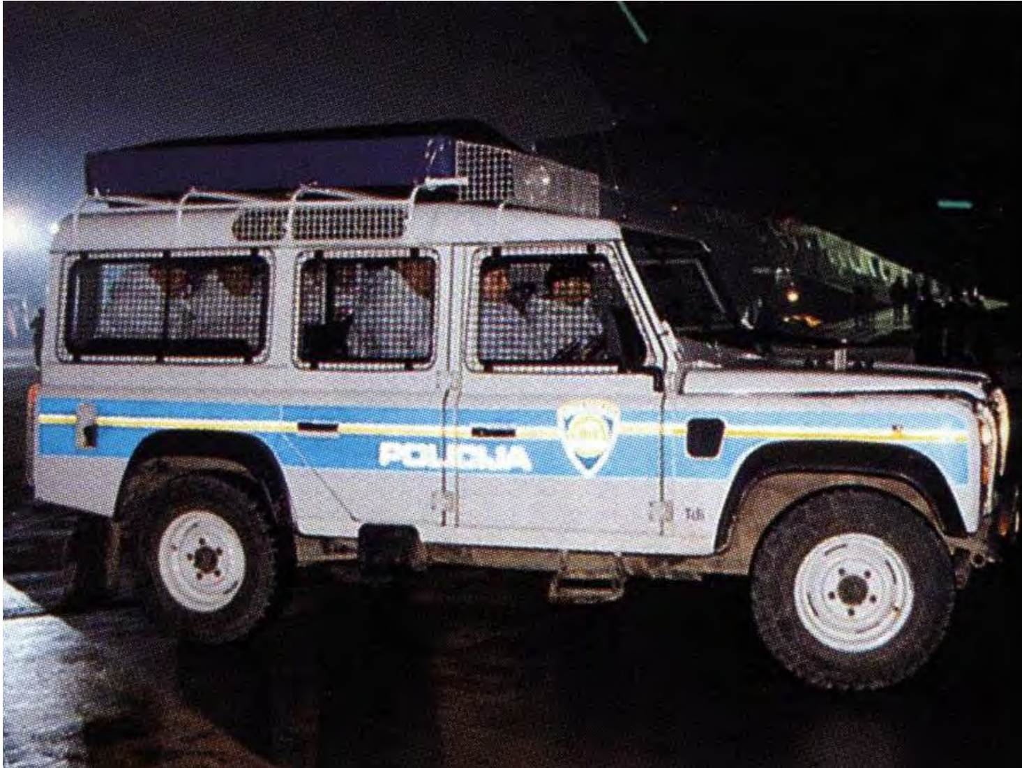
Land Rover Defender 110 TDI SW 4x4 sa žičanom zaštitom Land Rover Defender 110 TDI SW 4x4 with a wire mesh protection
