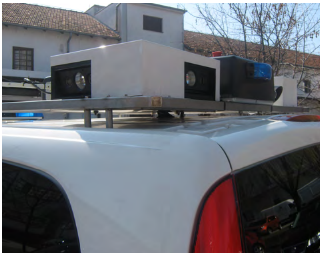
Pogled na unutarnji uredski prostor vozila, kamere i podizne reflektore na krovu vozila The look of the vehicle office interior, cameras and elevating spotlights on the vehicle roof
